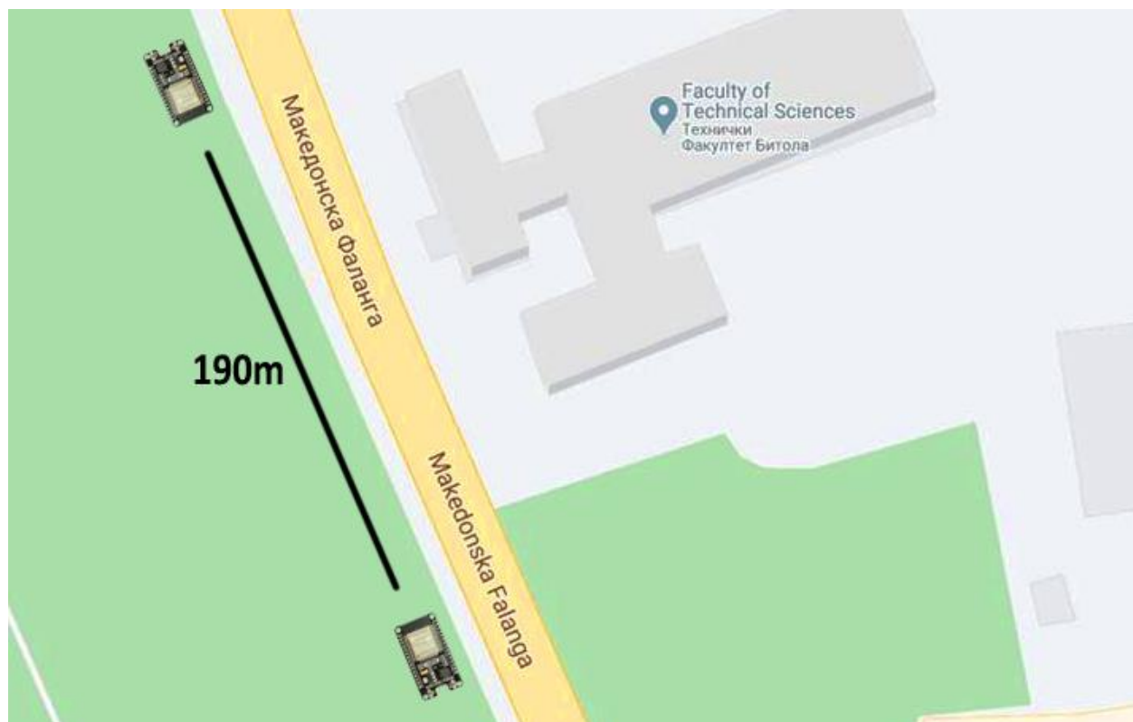
Figure 5. ESP-NOW communication range
